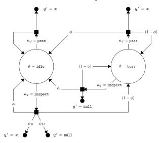
Fig. 2. Intrusion detector state transition diagram
